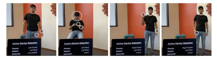
Figure 10: Active device tracking across different device combinations. Active devices are highlighted with a white circle for illustration and the foreground laptop shows the live tracking result.
