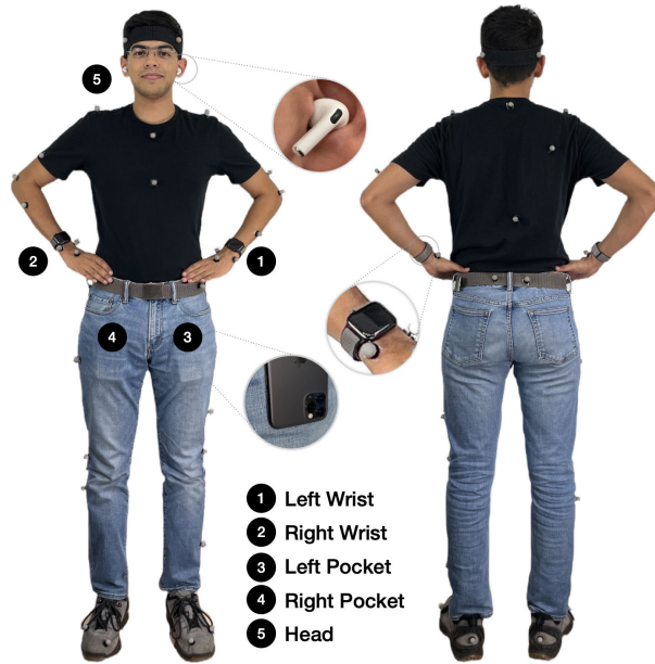
Figure 8.5: IMUPoser data collection setup. Participants wore 2 smartwatches, kept 2 smartphones in their front pockets, and wore wireless earbuds. 41 retroreflective motion capture markers were also placed around the body to track ground truth body pose.
