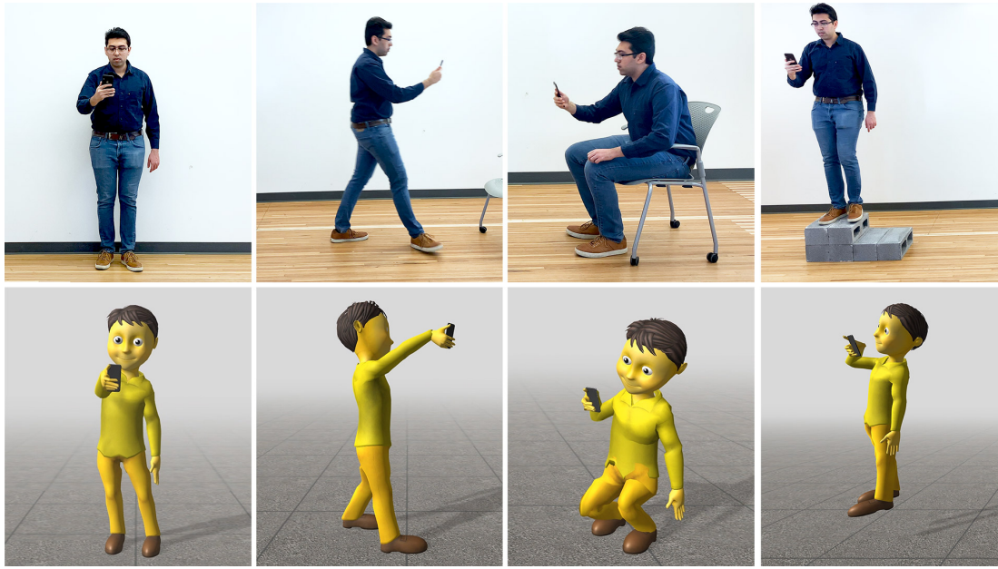
Figure 5.9: A user standing (far left), walking, (center left), sitting (center right) and standing on a box (far right) is mirrored by the avatar.
