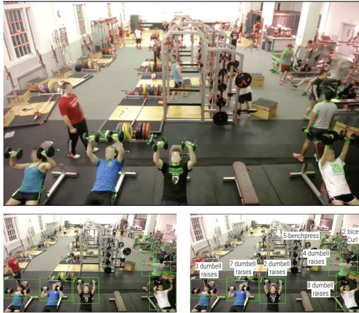
Figure 4.2: GymCam uses a camera to track exercises. Top: Optical flow tracking motion trajectories. Bottom Left: Exercises clustered. Bottom Right: Exercise Recognition.
