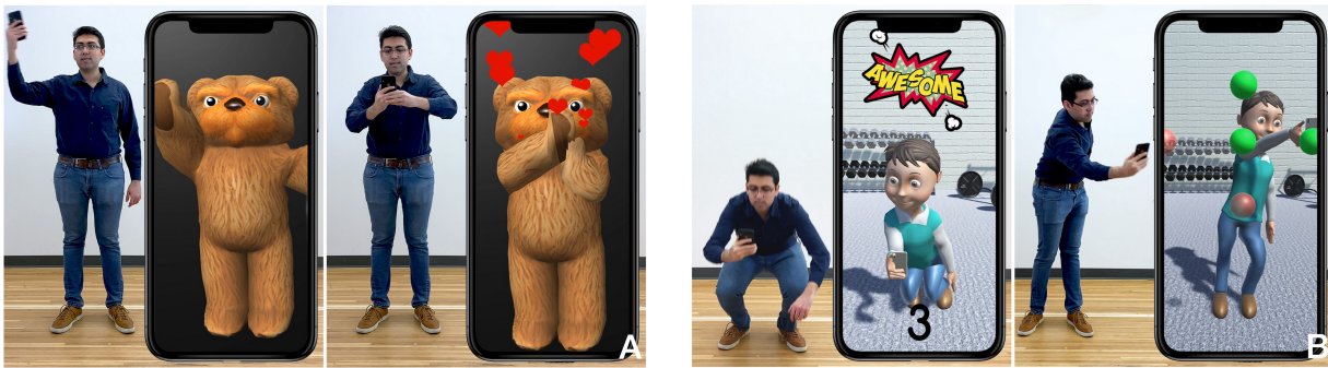
Figure 5.11: A) Full-body “Animoji” enabled by Pose-on-the-Go, where users can wave (left) and hug (right). B) A tool for health sensing such as counting squats (left) and reaching targets for physical rehabilitation (right).
