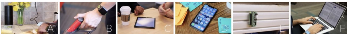
Figure 4.1: Ubicoustics enables real-time activity recognition across diverse hardware platforms, including smart speakers (A), smartwatches (B), tablets (C), phones (D), IoT sensors (E) and laptops (F).
