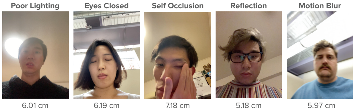
Figure 5.4: Example images where my RGBD Gaze model had high error. Euclidean error is noted below each image.
